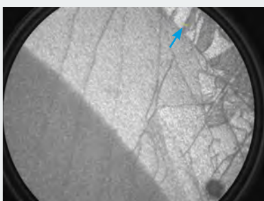
Bright-field LEEM image of MoS 2 on SiO 2 on Si taken (courtesy of J. Jobst). 7 μm field of view
