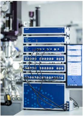
Nanonis Mimea setup taylored for a SPECS Aarhus 150 NAP Scanning Probe Microscope
