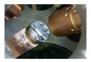
Sample holder stage with SH 2/12 sample plate inside FlexPS module in front of electron spectroscopy equipment
