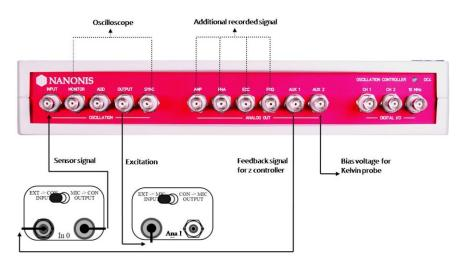
Fig. 2.Schematic of the connection of the Nanonis OC4-Station to EnviroScope via the SAM box.
