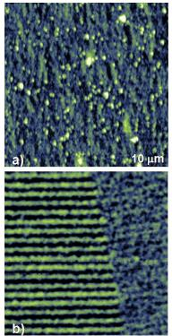
Fig. 1. MFM measurements on standard magnetic tape sample in high vaccum 1E - 6 mbar. a) topography, b)  $\Delta f$  signal on the second pass at 100nm above the surface.
