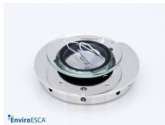
Fig. 1 Typical set-up with a solid sample in solution for solid-liquid interface studies using the EnviroESCA.
