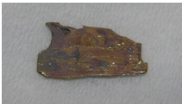
Fig. 1 Studied single crystal of vanadium pentoxide (V 2 O 5 )
