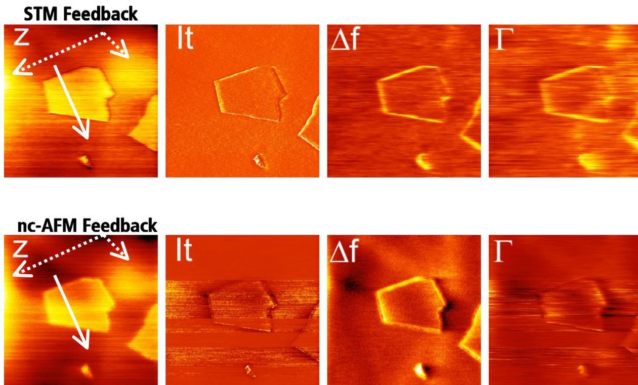
**Figure 4: Imaging of the same area on the HOPG surface in STM and nc-AFM feedback mode**
