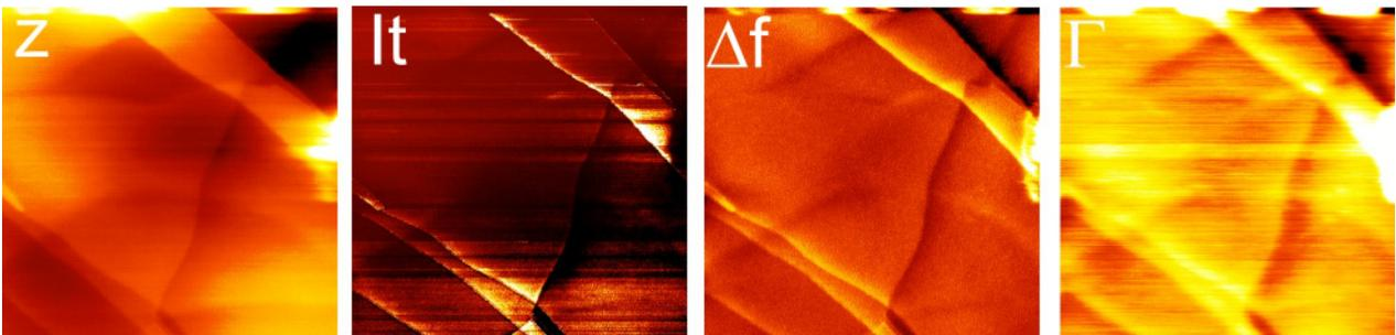
**Figure 3: Imaging of the same area on the HOPG surface in STM and nc-AFM feedback mode**
