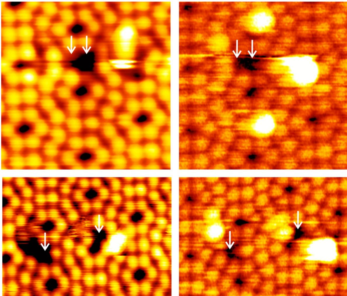
**Figure 2: Identification of defects on the surface by combined imaging with STM and nc-AFM**
