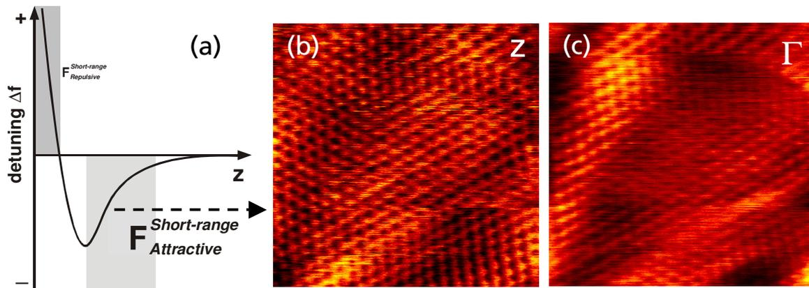
**Figure 6: Atomic-resolution NC-AFM imaging on Au(111) in the attractive regime**
