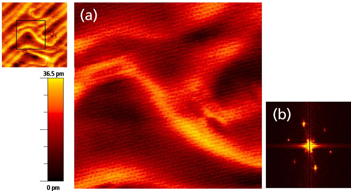
**Figure 4: Atomic details of the herringbone reconstruction imaged by NC-AFM**
