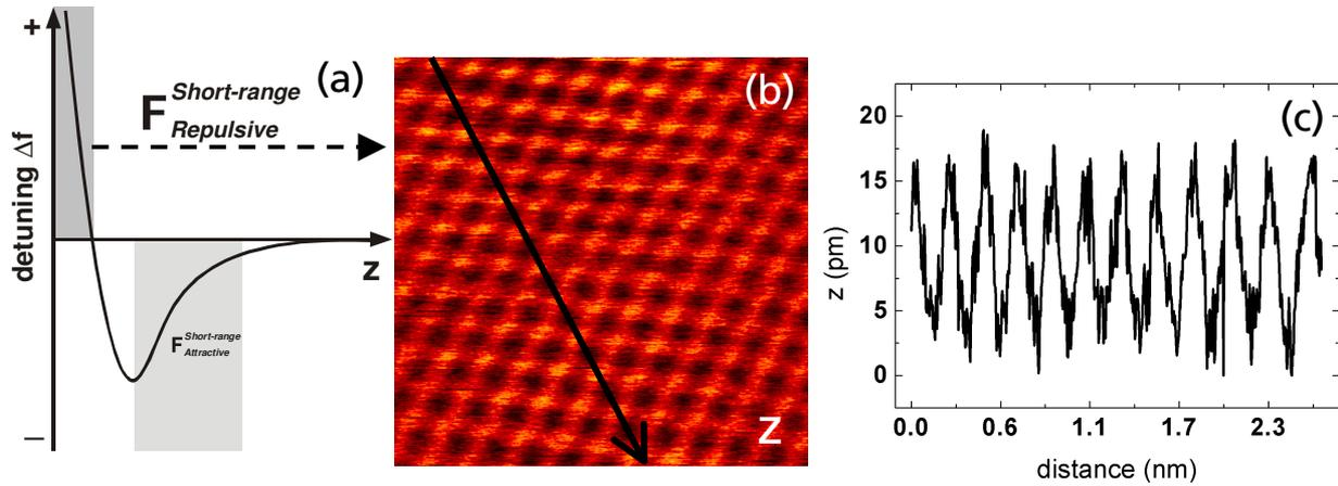
**Figure 5: Atomic-resolution NC-AFM imaging on Au(111) in the repulsive regime**
