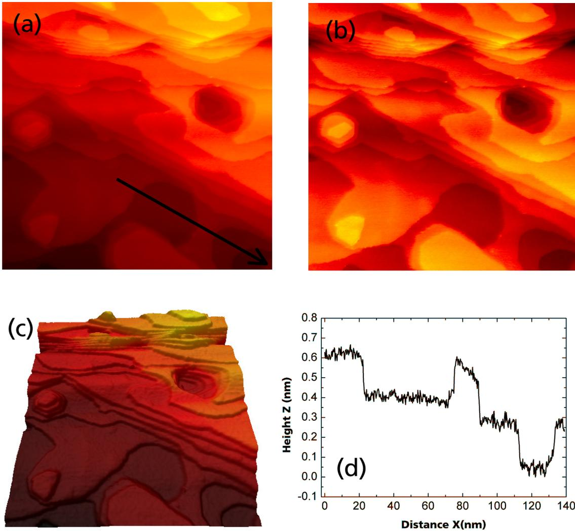
**Figure 1: Large scale NC-AFM image of the Au(111) surface**
