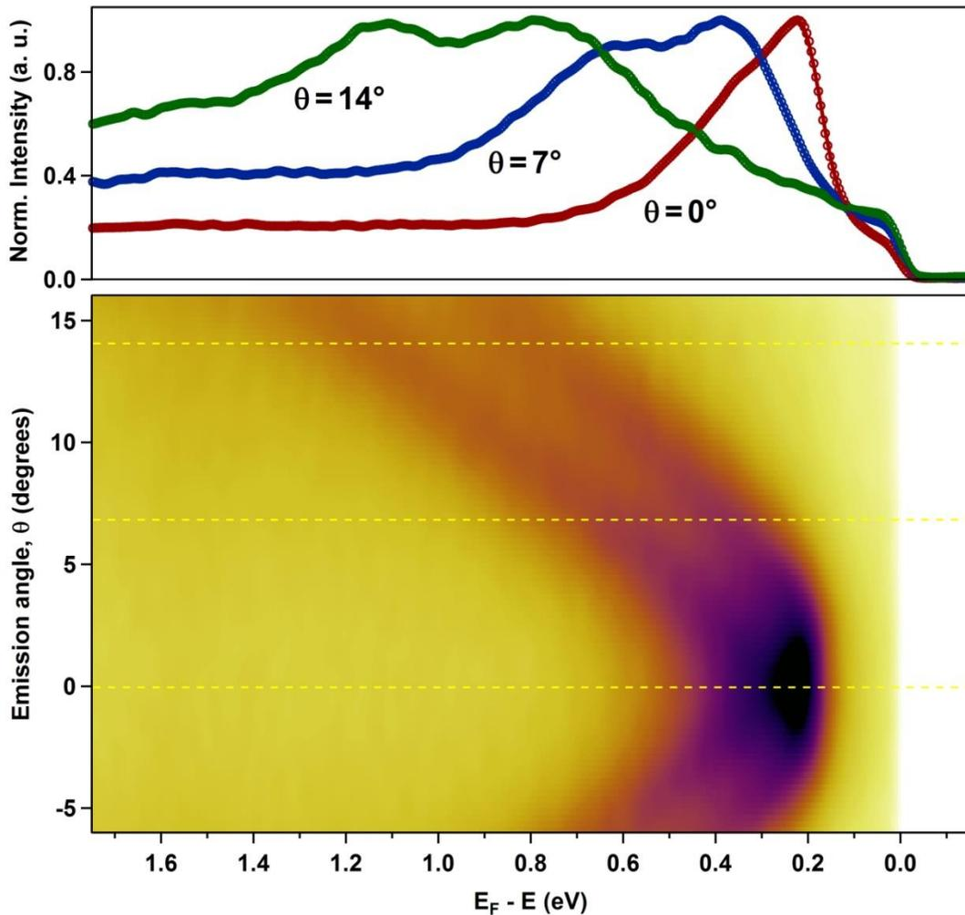
Figure 4: Photoelectron intensity 2D map obtained in normal emission geometry with XeI UV emission line for the graphene/Ir(111) sample. The Rashba split Ir surface state is clearly resolved. Upper panel shows representative spectra extracted from the intensity map for the emission angles  $0^\circ$ ,  $7^\circ$ , and  $14^\circ$ , respectively (emission angles are marked by the dashed lines on the lower panel).
