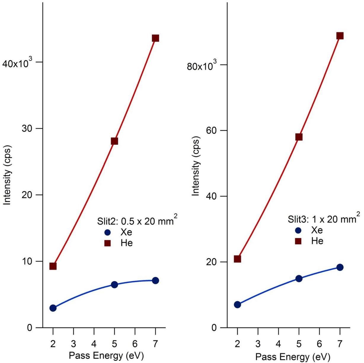
Figure 3: Extracted photoelectron intensity measured on the polycrystalline Ag sample. Raw data are presented in Fig. 2. All points correspond to the binding energy of 0.15eV.
