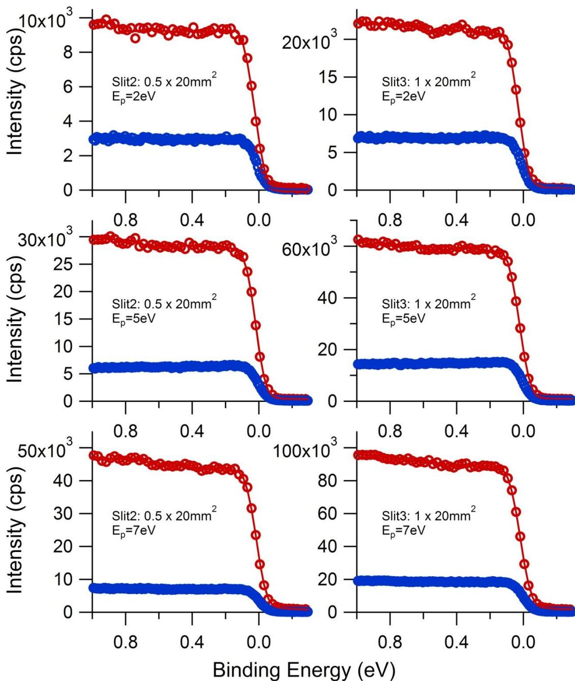
Figure 2: Angle-integrated photoelectron spectra of the polycrystalline Ag sample measured in the vicinity of the Fermi level with HeI (brown symbols) and XeI (blue symbols) ultraviolet light. These measurements were performed for two entrance slits: #2 ( $0.5 \times 20\text{mm}^2$ ) and #3 ( $1 \times 20\text{mm}^2$ ) and different pass energies of the analyzer,  $E_p$ . All spectra were recorded at room temperature of the Ag sample.
