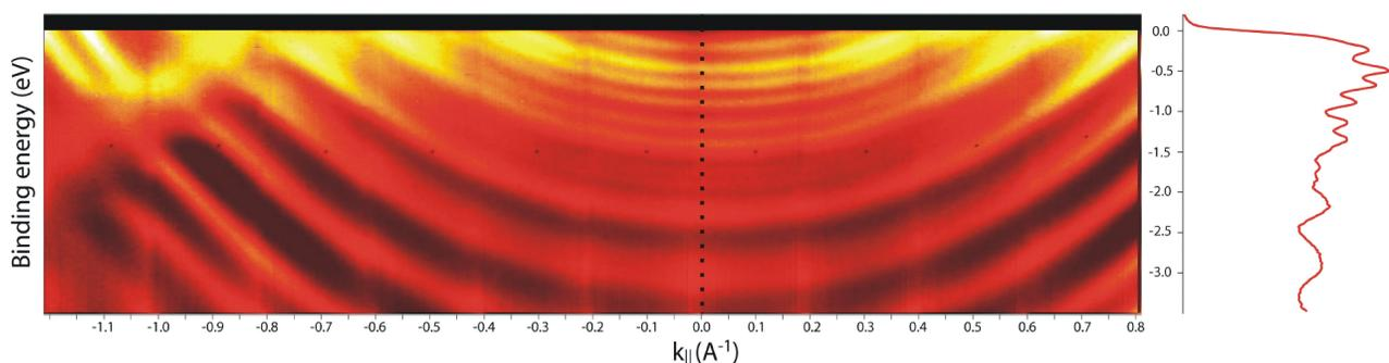
The Photoemission intensity distribution as a function of the binding energy and the parallel component of the wave vector from a nominal nine monolayers thick Al-coating on a single-crystal Graphite layer on SiC(0001). The measurements were carried out with a photon energy of 15 eV at BESSY in Berlin and a SPECS PHOIBOS 100 2D-CCD Analyzer. Data courtesy J.H. Dil, Th. Kampen, K. Horn (Fritz Haber Institute, Berlin)
