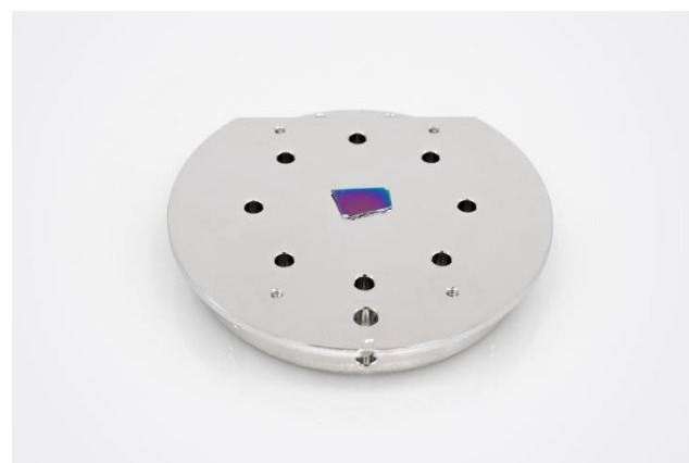
Fig. 1 Sample of an organic thin film coated on silicon used for sputter depth profiling with argon gas clusters
